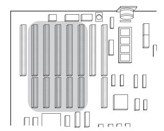
Figure 62. Computer Expansion Slots for installing an ISA Buffer Card
